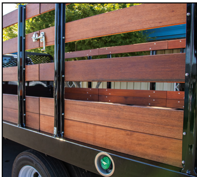
Flatbar Rail and Flatbar Supports 2" x 3/8"
