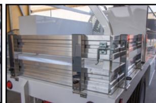
15" Fold Down Side Racks With Aluminum Slats and Stainless Steel Stakes
