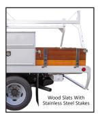
• Removeable 3" x 2" x 120" wall with 2" legs and 3" x 2" removeable crossbars
