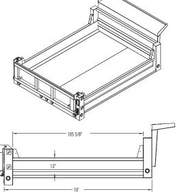
NOTE: 13" DIMENSION IS FROM FLOOR TO TOP OF SIDE RAIL
