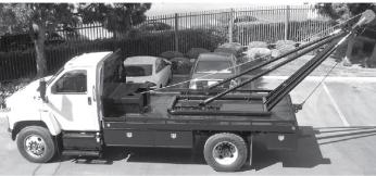
A 13 ft or 15 ft long A-Frame body with crane. Diamond plate 3/16" steel, cab high headboard, tubing for side racks, custom tail plate with two vise racks, diamond plate steel covering winch, kill switch, back up alarm, pintle hitch, multiple tool boxes.
