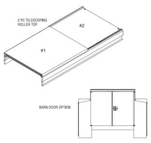
Roller Tops come with stainless steel track and rollers.
