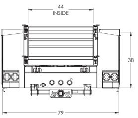
Dimensions for SB-98-79-49-38-VO 2 CUBIC YARD DUMP INSERT
