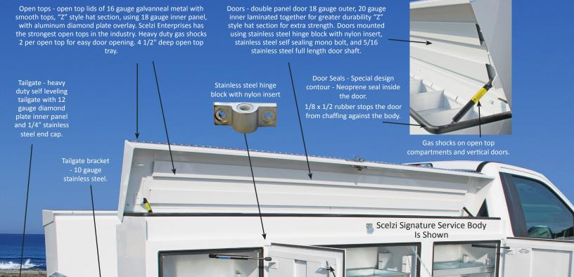
Tail hinges on 5/8" stainless steel Allen Head Shoulder Bolt Bushing.
