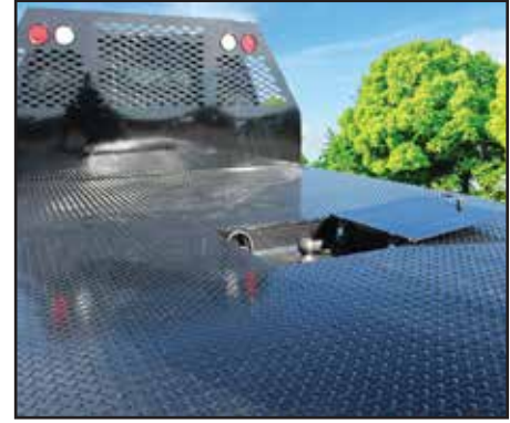
Integrated gooseneck hitch with 2-5/16" ball plus side flip lid.
